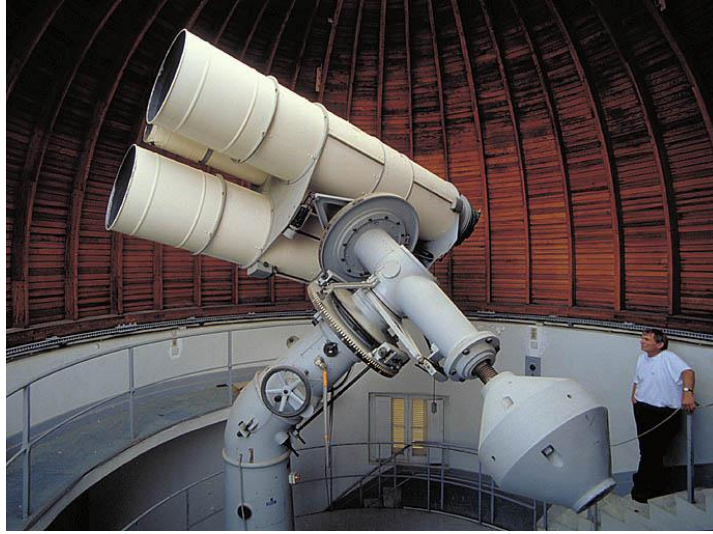
Figure 1: The Zeiss binocular astrograph at Observatoire de Nice . (Marc Heller © OCA).
