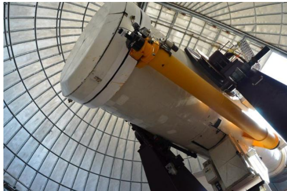
Figure 2: TESCA, the Calern observatory Schmidt telescope. (© OCA).
