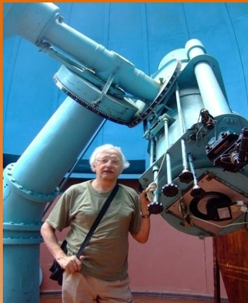
40 cm astrograph, SAI Crimean Station. Field  $10 \times 10^\circ$ , scale  $120''/\text{mm}$ , exposures of 45 min, plate limit  $\sim 17$  mag
